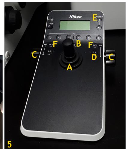
Using the focus wheels on the side of the Nikon controller box (Fig. 5C), move the objective nosepiece up until your sample is in focus (towards you = up, towards the wall = down). Switch to 'Fine Focus' by clicking on the 'Z' button on the controller box (Fig 5D). Fine and coarse focus are also indicated on the display (  $\wedge$   $\hat{\wedge}$  ).
